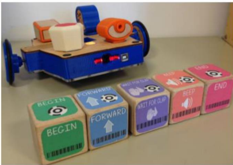
Figure 12. KIWI robotics kit combined with the tangible programming language CHERP, Sullivan et al. (2016)
